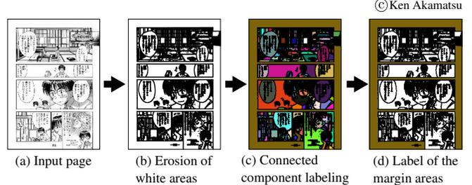
**Fig. 3.** (a) An input image. (b) Erosion is applied to white regions to thicken the lines. (c) White-connected areas are labeled with the same value. (d) The margin areas are selected.
