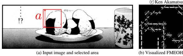
**Fig. 2.** (a) An image and a selected square area.  $a$  measures the side of the feature. (b) The visualized FMEOH feature extracted from the red selected area in (a).
