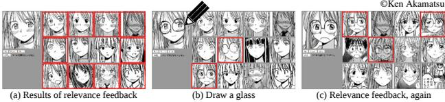
**Fig. 7.** Query retouch. (a) Results of relevance feedback where target characters are red colored. (b) The user adds strokes and draws a glass with the target character. Another target characters with a glass are then retrieved (colored red). Note users can erase lines using an eraser tool. (c) Both relevance feedback and query retouch can be conducted multiple times.
